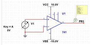
The input signal is a DC\_INTERACTIVE\_VOLTAGE. Set it to a Maximum value of 0.1 V and a Minimum value of -0.1 V, and set the increment to 0.5%. Run the simulator, and see if you can get anything other than some maximum value (around 9 V) and a similar minimum value (around -9V).
