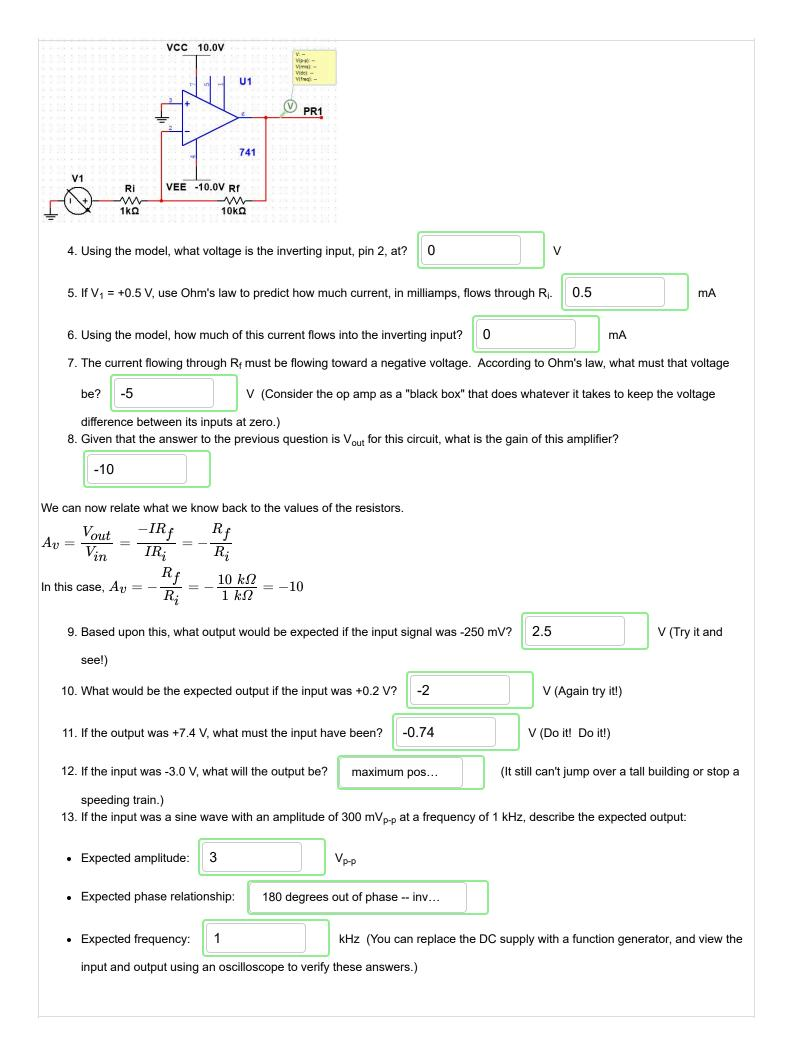
In the next lesson, we'll revisit this amplifier and develop the standard characteristics expected for some other standard op amp circuit configurations.
