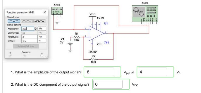
If all went well, you should have discovered that, even though the input signal has a large DC offset, the output signal does not. Let's analyze the circuit to understand why.
