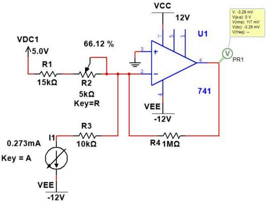
Set the current source to 273  $\mu$ A, then adjust the potentiometer until the output is a close as possible to 0 V.
