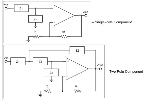
In each case, the "Z" elements are either resistors or capacitors. Z1 and Z3 have to be the same type of component, and Z2 and Z4 have to be the other type of component. If the odd-numbered ones are resistors, the result is a LPF. If the odd-numbered ones are capacitors, the result is a HPF.
