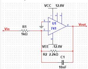
Quick analysis: this is an inverting amplifier, and the capacitor in parallel with the feedback resistor makes it a Low-Pass Filter (LPF). Its passband gain would be  $-2.2k\Omega/1.0k\Omega = -2.2$
