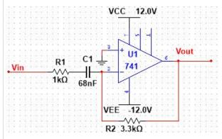
Quick analysis: this is an inverting amplifier, and the capacitor in series with the input resistor makes it a High Pass Filter (HPF). Its passband gain would be  $-3.3k\Omega/1k\Omega = -3.3$
